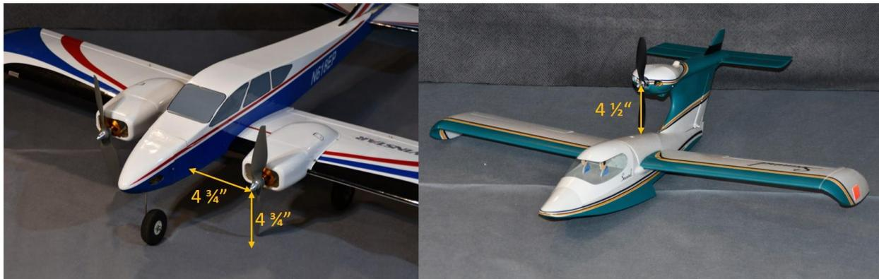
Figure 3: Examples of significant ground and/or fuselage propeller clearance limitations
